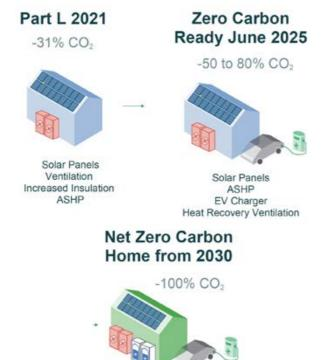
Figure 6.31 - Potential sustainability path to Net Zero Carbon homes 2030. The range of measures used will be addressed at the Reserved Matters stage
